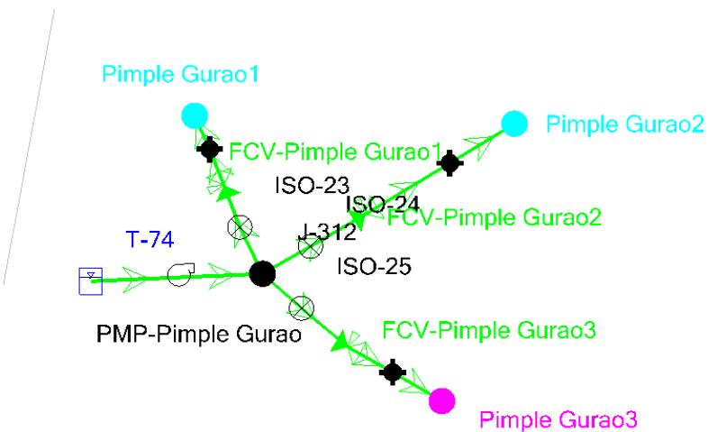
Figure 6.15: Pumping at ESR Sector 28 New with sump
