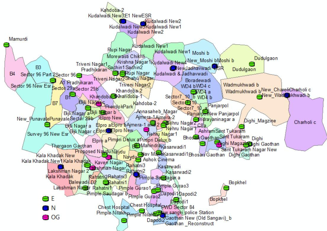
Figure 6.1: Existing (E) ongoing (OG) and new (N) tanks proposed
