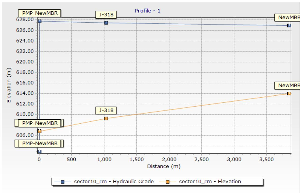
Figure 6.7: Profile of pressure from the sump to the new MBR
