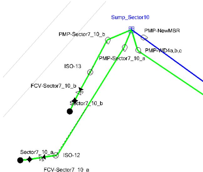
Figure 6.5: Details of pumps at sump at Sector 7,10
