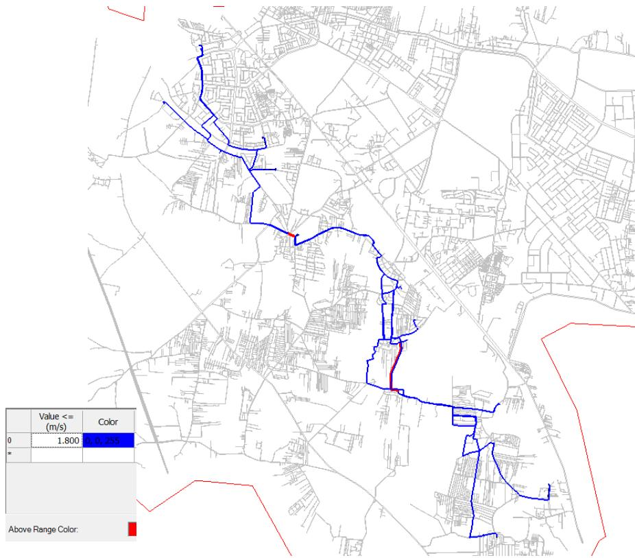
Figure 6.21: Velocity in gravity pipeline of Chinchwad
