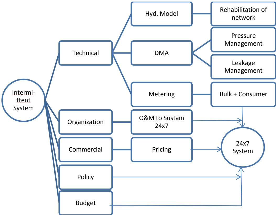
Figure 5.1: Road map of 24/7 continuous water supply
