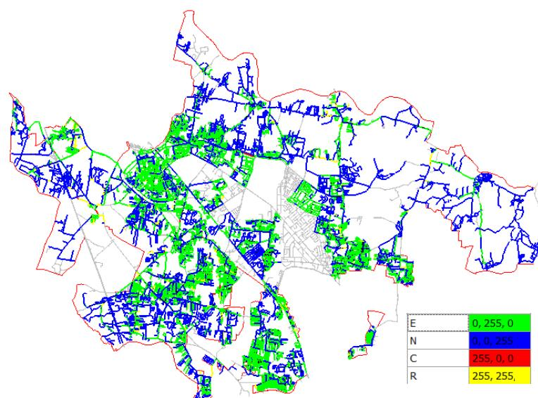
**Figure 7.2:** All pipelines (existing and new) in the distribution network
