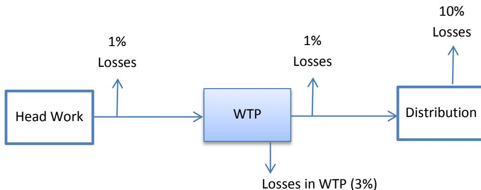
Figure 4.1: Demand of en-route connections and losses in WTP
