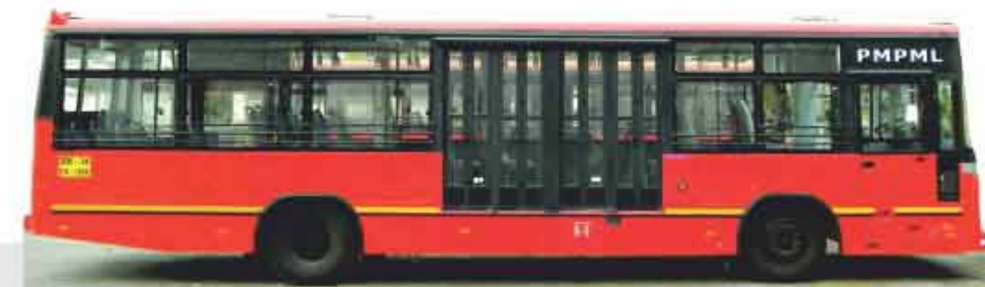
The wide doors on the right side help more passengers to board or alight in limited time at BRT stations
