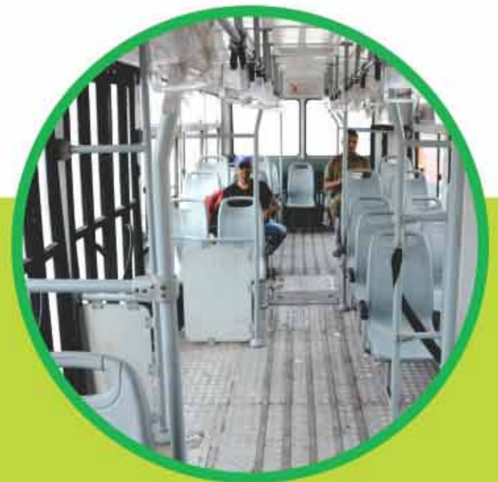
The wide doors on the right side help more passengers to board or alight in limited time at BRT stations
